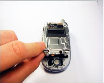
Gently loosen the second protective cover with the plastic opening tool.
