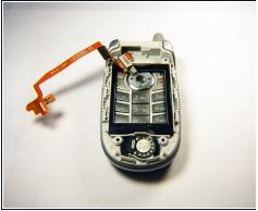
• Gently slip the copper strip out from under the circuitry by using your hand.
