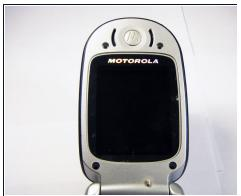
On the phone's face, remove the four rubber caps from the screw covers using a <u>spudger</u>.
