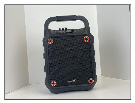
Remove the four screws from the outer cage of the speaker using a Phillips #00 screwdriver.
