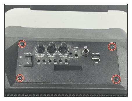
Remove the four screws from the top panel of the controls using a Phillips #00 screwdriver.
