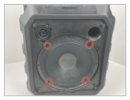
Remove the four screws from the outer edge of the speaker using a Phillips #00 screwdriver.
