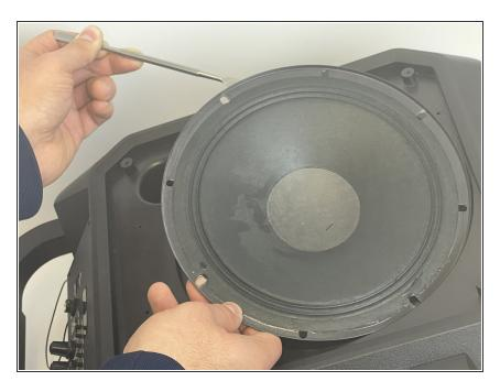
Using a prying tool, gently remove the subwoofer from its hole.
