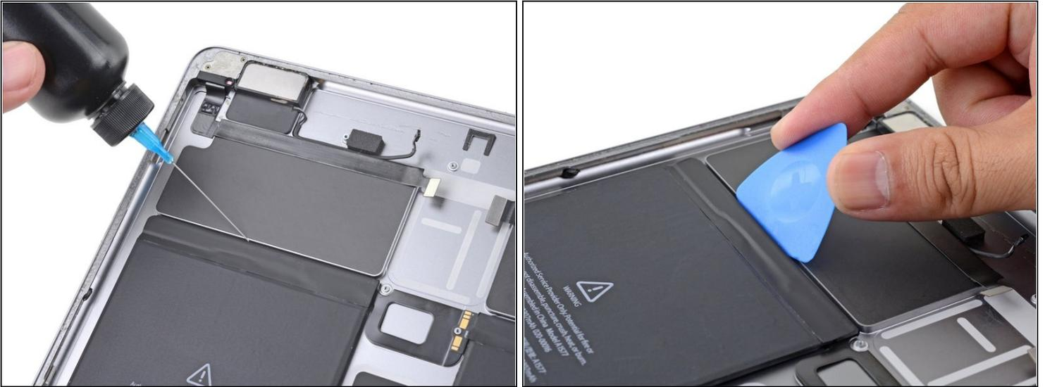
① Repeat the procedure for the top left edge of the battery:
