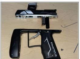
Remove the two main screws using a 2.5 mm Allen key to separate the air transfer plate from the frame.
