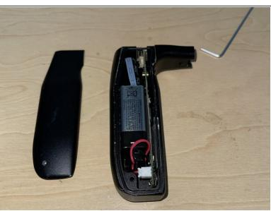
Use a 1.2 mm Allen key to remove the screw, and remove the cover to expose the OLED Board.
