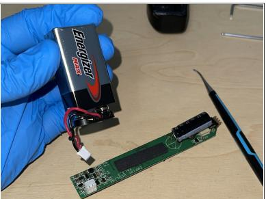
Disconnect the battery from the OLED board.
