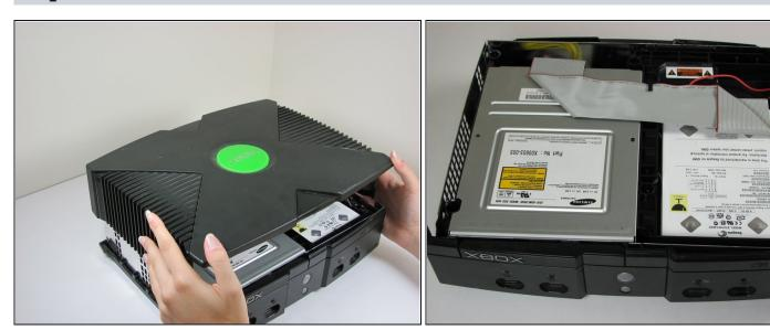
• Once the bottom and top shells are no longer attached, carefully turn the Xbox right-side-up, lift and remove the top cover.
