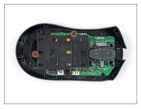
Use a Phillips screwdriver to remove the two 3.4 mm screws securing the battery housing to the bottom half of the mouse.
