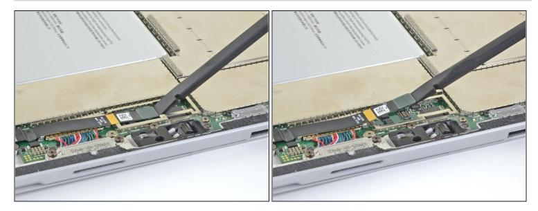
• Use the flat end of your spudger to lift the microSD card reader's connector straight up out of its socket.
