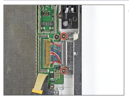
Use a T5 Torx screwdriver to remove the two 3.7 mm screws securing the charging assembly.
