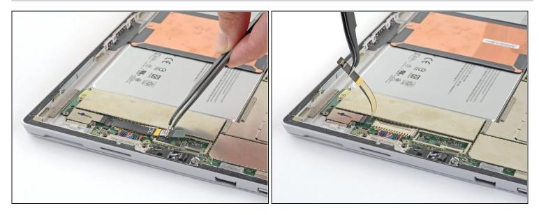
• Lift the microSD card reader cable up and out of the way of the EMI shield covering the charging assembly.
