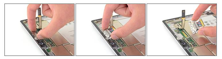
• Tilt the back of the charging assembly up to about a 30 degree angle and pull it straight back out of the chassis.
