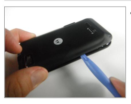
Once wedged in the opening, gently pry around the phone until back cover lifts off.
