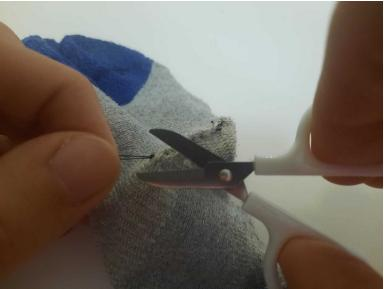
Cut the excess thread with the scissors.
