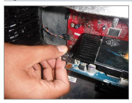
Unplug the cable labeled "P3" on the left side of the graphics card. Be sure to push the plastic pin all the way down and pull firmly.
