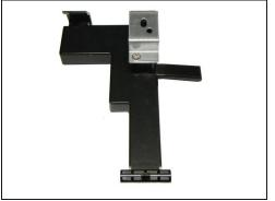
• Remove the support underneath the processor cooler by pressing down on the latch at the top of the support and pulling the support towards you.
