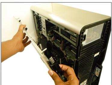
Remove the cover panel on the side of the computer by pulling out the latch on the back panel and pulling the panel downwards towards the ground.
