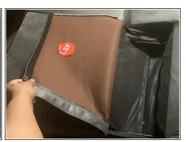
Remove the snap cover that is covering the back to show the seat's sliding mechanism.
