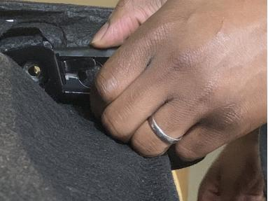
Align the hole of the sliding mechanism to hole on the wood of the seat.
