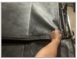
Cover the sliding mechanisms with the snap cover.
