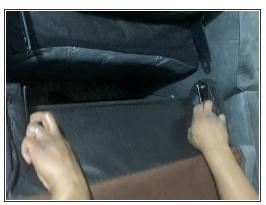
Pull off the seat connected to its base by pulling the clamps on both sides outward and the seat towards your body.
