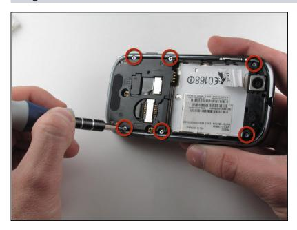
Remove the six 4.0 mm T4 Torx screws which line the edge of the back of the phone.
