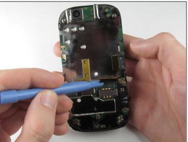
Pry the orange keyboard connector from its socket on the motherboard using the edge of the plastic opening tool.
