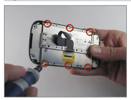
Remove the six 3.0 mm T4 Torx screws that align on the phone's sides.
