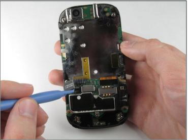
• Wedge the plastic opening tool underneath the black display connector and pry it off its socket on the motherboard.
