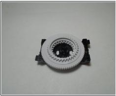
• Disassemble the adjuster assembly spring, small gear, large gear, and bracket in order to replace the broken component.
