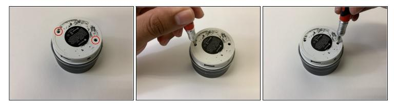
• Remove the two bottom screws using a Phillips #0 screwdriver.
