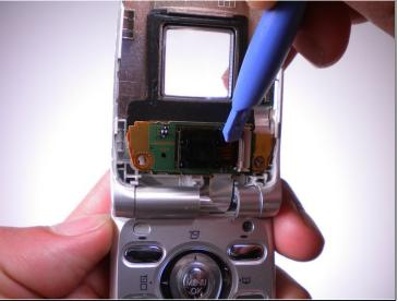
Use the plastic opening tool to flip the ZIF connector to the right.
