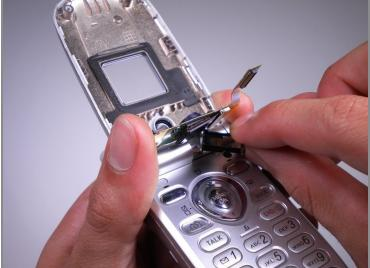
Use the opening tool to take off the black plastic frame around the camera lens.
