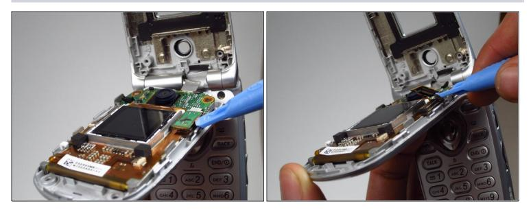
Use plastic opening tool to lift the chip on the right side.
