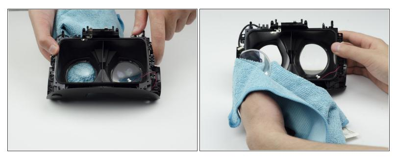
Using a glass cloth (or any cloth with soft fibers), carefully press on the lenses until they pop out of place.
