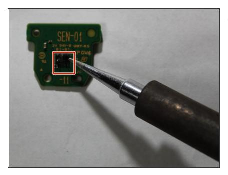
Desolder the faulty infrared range finder from the backside of the board.
