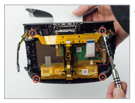
Unscrew the four silver 6 mm screws in each corner using a PH #000 screwdriver.
