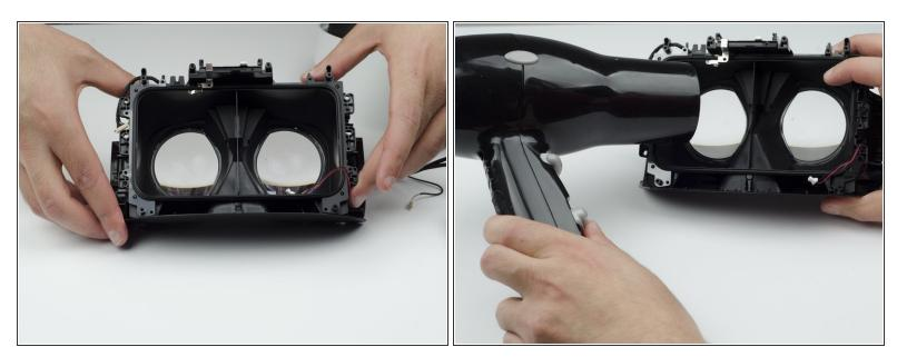
• Using a hairdryer (or heatlamp), warm the area around the lenses. This will help loosen them for removal.
