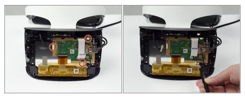
Using the tweezers, unplug the three (one black bundled, two multi colored bundled) connector cables from their ports along the circuit board.
