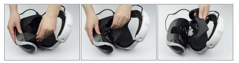
• Peel back the rubber covering around the lenses to remove the surrounding plastic eyepieces.
