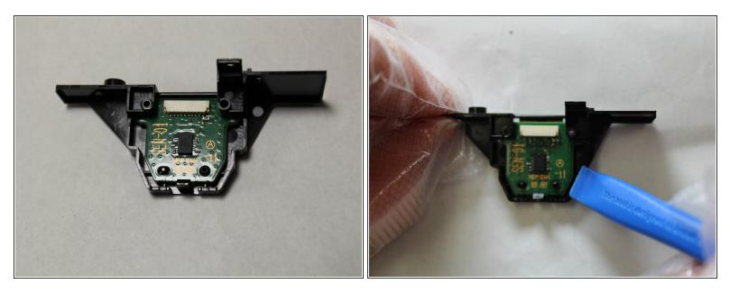
• Gently pry outward with an opening tool to remove the board from the bracket assembly.
