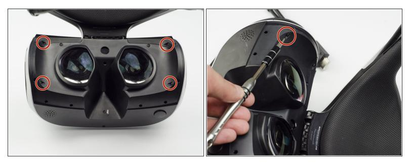
Unscrew four 13 mm screws with a PH #000 screwdriver.
