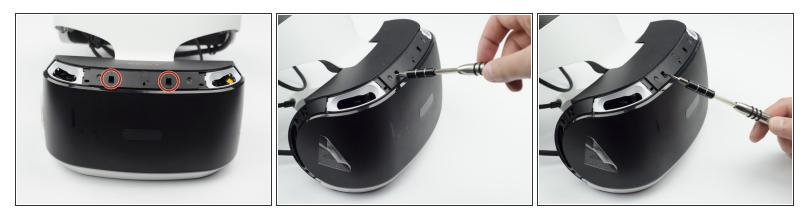
Unscrew the two 7 mm screws from the top of the headset.
