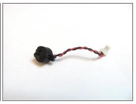
Twist the rubber casing and remove it from the plastic cover.
