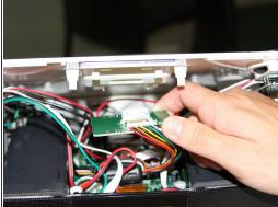
Unscrew the four black 7mm screws with the Phillips #1 screw driver that hold the middle circuit board to the top case.
