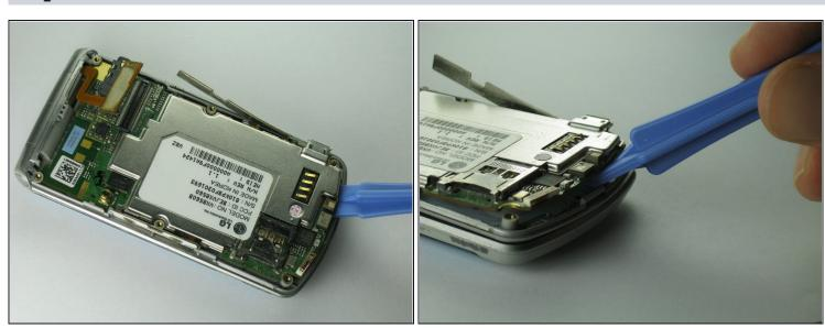
Carefully insert the plastic opening tool between the motherboard and the back of the phone.
