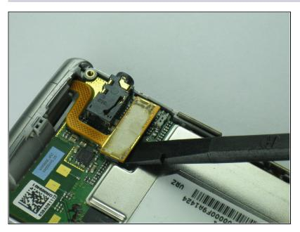
Use the flat end of the spudger to lift the orange display data cable.
