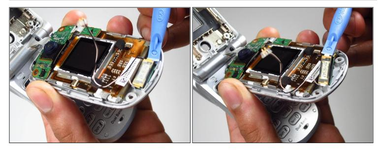
Use the opening tool to pull the earpiece off of the top panel.
