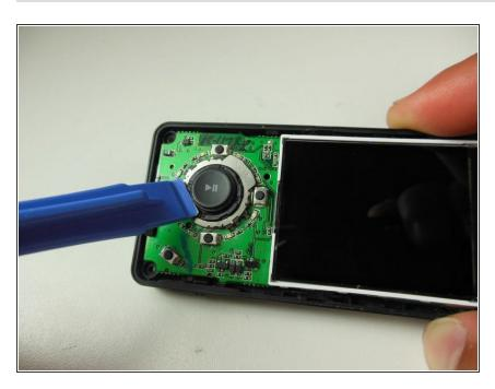
Slightly insert plastic opening tool underneath any side of the play button.
