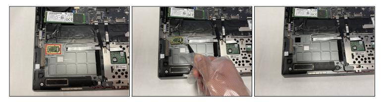
• Lift and remove the fingerprint reader from the laptop using the angled ESD tweezers.
