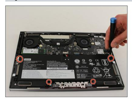
• Unscrew the four 3mm screws with a Phillips screwdriver.
