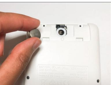
Remove the worn-out LR44 battery inside using a spudger.
