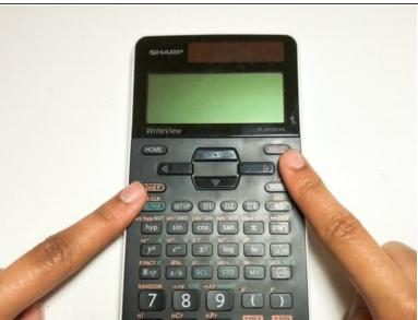
Turn off the calculator by pressing both the [2NDF] and [ON] buttons at the same time.
