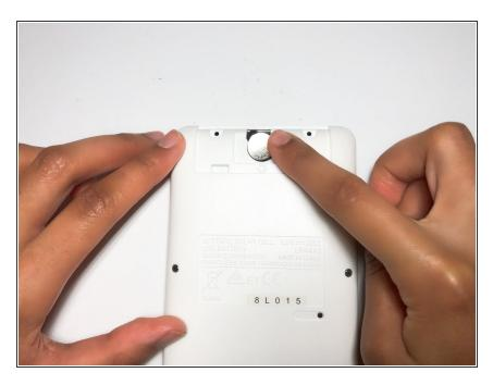
Gently insert the new LR44 battery in the empty battery slot.
