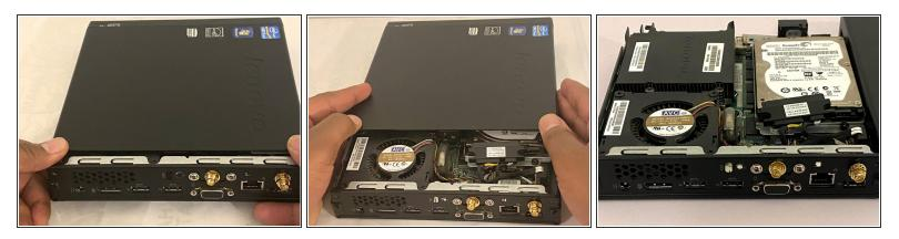
• Use your thumbs and slide the metal housing towards the front, to remove the cover.
