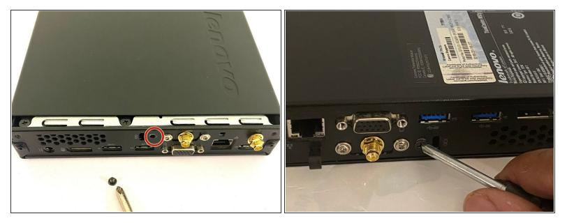
Using a Phillips #1 screwdriver, remove the middle black screw located on the back of the ThinkCentre.
