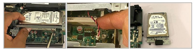
**Do not try to remove the hard drive right away** .There is a red/black cable connected to the motherboard, right below the hard drive. Gently disconnect it from the \*green\* motherboard\*\*\*.
