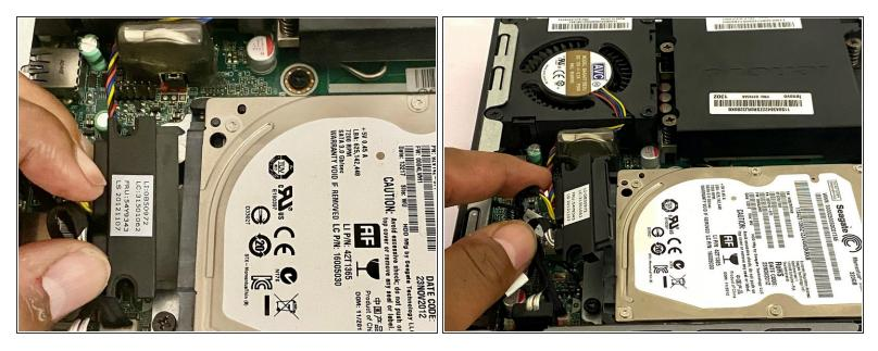
• Unplug the black connector from the damaged hard drive.
