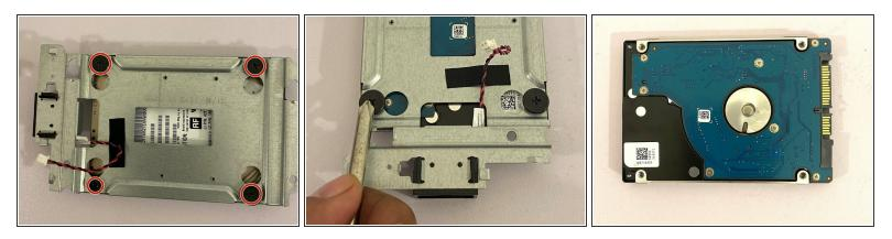
• Flip over the disconnected caddy/tray and use the Phillips #1 screwdriver to remove the four screws from the bottom. Then remove the hard drive.
