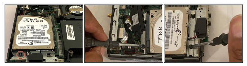
Use the Phillips #1 screwdriver to remove the two black screws holding the hard drive to the chassis.
