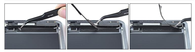
• Use a pair of tweezers to lift up the fourth left antenna cable sticker.
