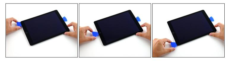
• Slide the left-hand opening pick along the bottom edge of the display, then remove it from the bottom right corner of the iPad.
