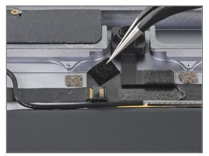
Use a pair of tweezers to remove the sticker covering the left ambient light sensor's ZIF connector.
