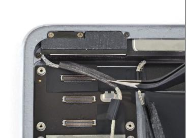
• Use a pair of tweezers to detach the large right antenna sticker between the logic board and the antenna.
