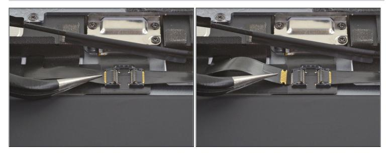
• Use a pair of tweezers to grip the left ribbon cable as close as possible to its contacts and pull the ribbon cable out of the ZIF connector.
