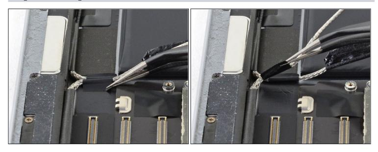
• Use a pair of tweezers to lift up the small sticker near the lower right speaker securing the right antenna to the frame.
