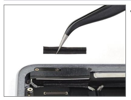
Remove the foam spacer from the second right antenna sticker.
