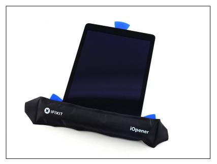
• Use the iOpener to apply heat to the bottom edge of the iPad.
