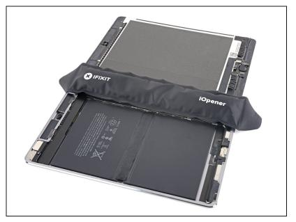
Apply a <u>heated iOpener</u> to the EMI shield on the logic board for one minute.
