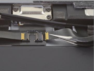
• Use a pair of tweezers to grip the right ribbon cable as close as possible to its contacts and pull the ribbon cable out of the ZIF connector.
