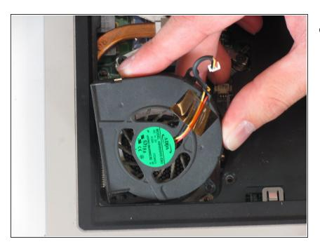
Take out the fan by lifting it out of its dock.
