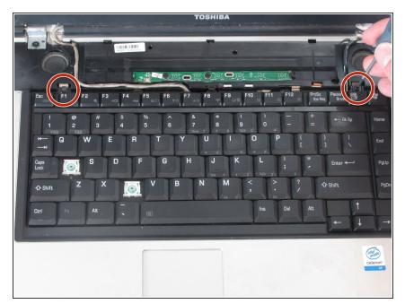
Remove the two 5mm Phillips #1 screws which hold the keyboard in place.
