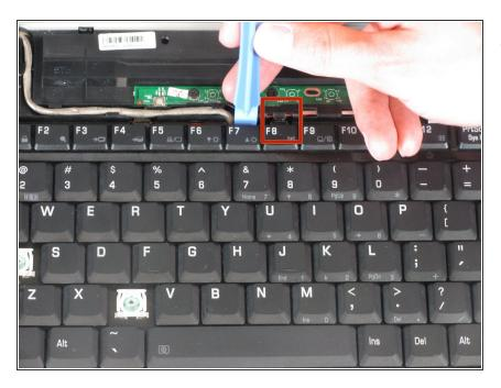
Unhook the plastic tab at the top of the keyboard using the plastic opening tool to pry the top of the keyboard up.
