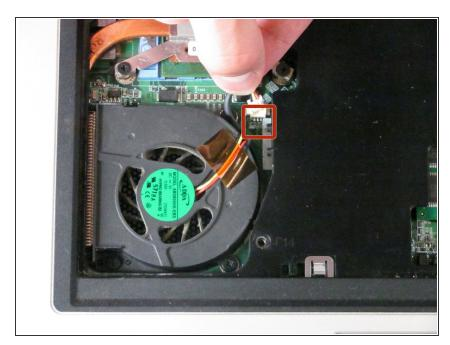
Pull the end of the white wire clip out of its port.
