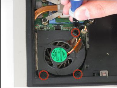
Locate and Remove the three 5mm Phillips #0 screws.
