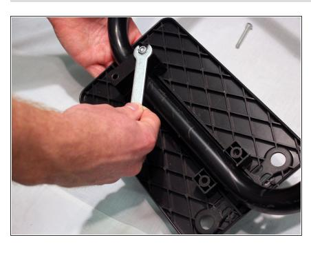
To remove the footrest, turn it upside-down and use the 10 mm box wrench to take out all four of the screws.
