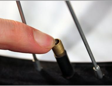
Release any air that remains by pressing down on the piston in the head of the stem.
