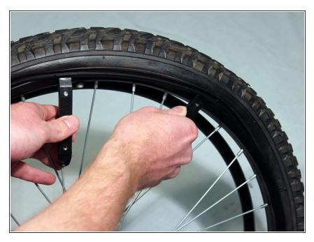
Holding one tire lever in place, slide the other lever around the rest of the wheel until the side of the tire is completely free of the rim.
