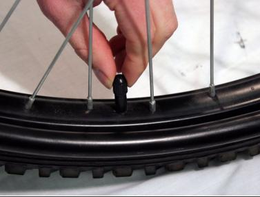
Unscrew the cap of the tube stem and set it aside.
