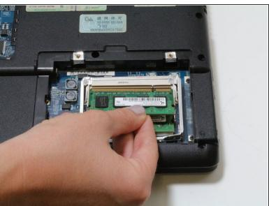
After the old RAM has been removed, insert the new RAM stick and ensure that they are oriented in the correct direction before installation. This can be done by lining up the gold connections to each other.
