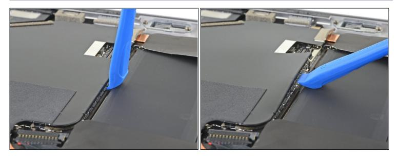
⚠ Be careful not to puncture or deform the battery with your opening tool.
