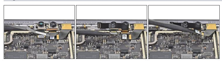
• Use the flat end of a spudger to pry up and disconnect all three camera connectors from the motherboard.
