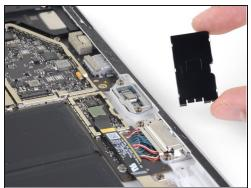
• Use an opening tool to pry up on the edge of the EMI shield covering the microSD card reader connector and remove it from the motherboard.
