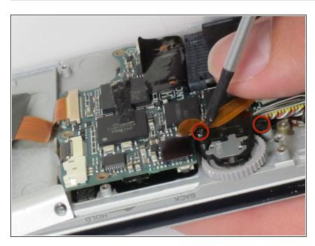
Lift up the orange ribbon cable and unscrew the two 2.5mm screws located at the corners of the audio module with a Phillips #00 screwdriver.
