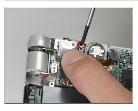
Unscrew the 2.5mm screw on the top portion of the audio module with a Phillips #00 screwdriver.
