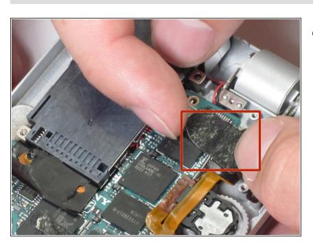
Remove the tape that is holding the module down.
