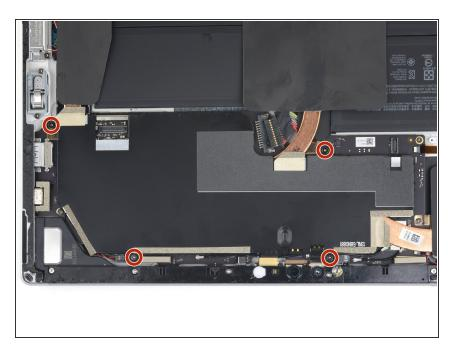
Use a T3 Torx screwdriver to remove the four 2.4 mm screws securing the EMI shield.
