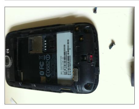
Put the bottom cover back in place and then replace all the screws
