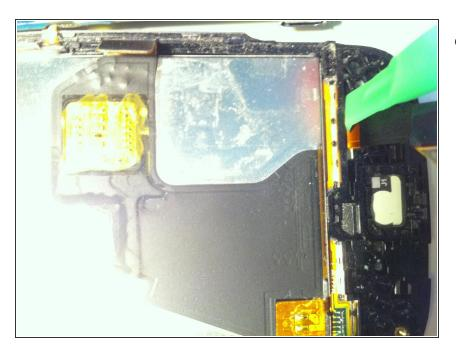
To detach the screen it can help to use a pry tool to push the screen from behind through the slot
