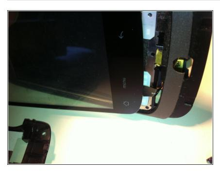
Once the connecter is pushed through the slot, you should now stick the new screen into place using suitable adhesive strip
