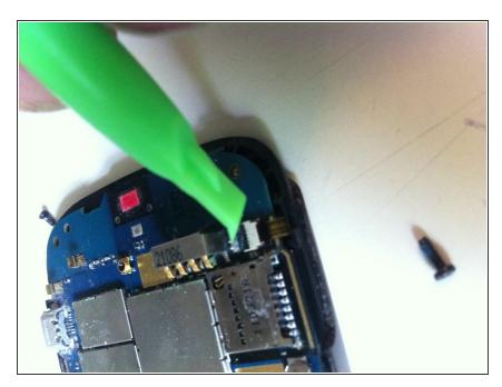
Reinsert the ribbon connector on the left hand side and push down the retaining catch
