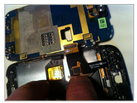
Fold down the ribbon connector from the screen and carefully fold the two casing halves together again, making sure that the two connectors are sticking out of the side
