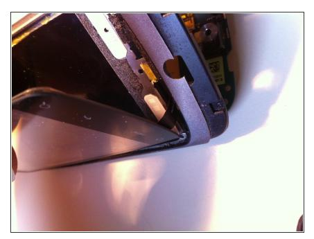
The screen is detached and the connector can be wiggled out through the slot
