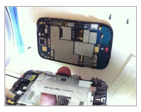
Clip the rear casing back on to the body
