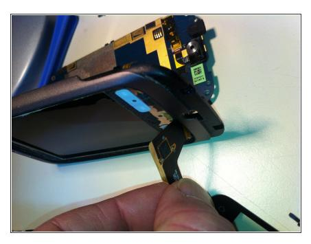
The connector for the new screen now has to be wiggled back through the slot
