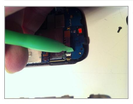
Lift up the retainer using a plastic opening tool.
