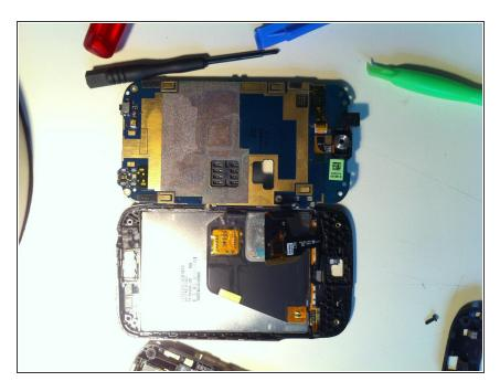
Carefully lift up the board from the left-hand side allowing it to 'hinge' on the metallic ribbon connector you have just noted and allow it to lay flat
