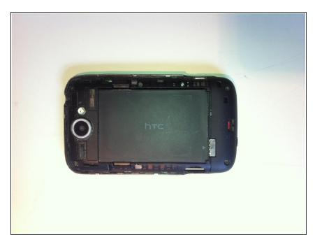
First remove the rear case/battery cover
