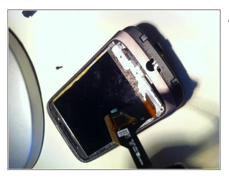
Remove the old screen and connector altogether
