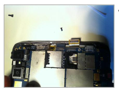
Reconnect the two connectors on the right hand side by pressing down
