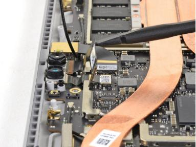
• Use the flat end of a spudger to lift the front camera ribbon cable off of the front camera connector.
