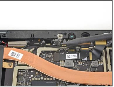
Use the pointed end of a spudger to pry up the connector next to the front-facing camera and disconnect it.
