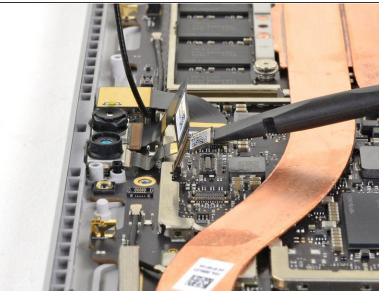
Use the flat end of a spudger to pry up the front-facing camera connector and disconnect it from the motherboard.
