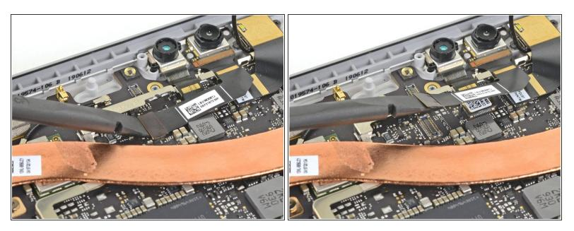
Use the flat end of a spudger to pry up the Hello face camera connector and disconnect it from the motherboard.
