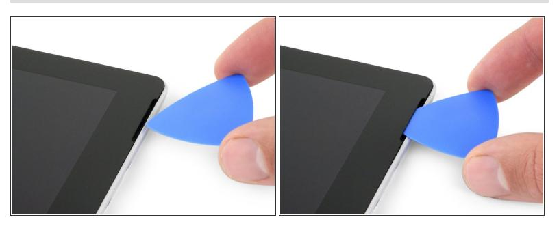
Insert an opening pick into the speaker opening on the screen and slide the pick between the glass and speaker grille.
