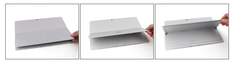
Lift the kickstand to expose the hinge screws.
