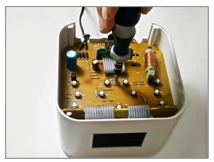
Using a Phillips #1 screwdriver, remove the screw found in the middle of the board.
