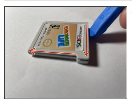
Go around all parts of the cartridge and do not crack the plastic.
