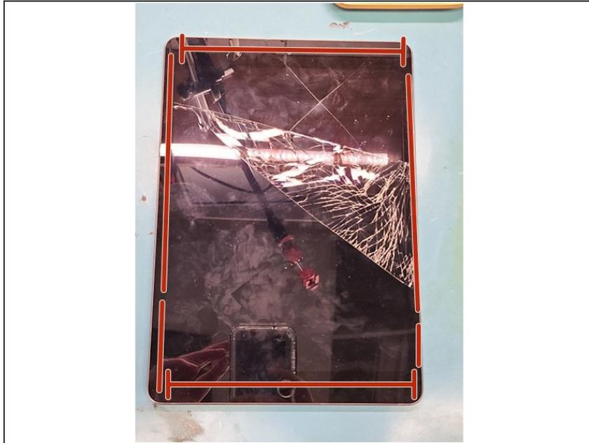
**⚠️** Apply heat to the screen (along the red lines), my personal rule is that hot to the touch is the best level of heat in order to weaken the adhesive. (Although not too hot).
