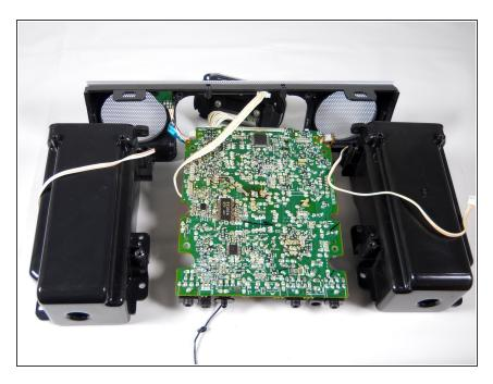
Disengage the clips on both sides of the speaker grille to separate the speakers from the rest of the assembly.
