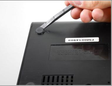
Slide a spudger under the two front rubber pads to expose two hidden screws.
