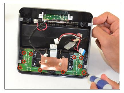
Unscrew the ten 6 mm Phillips #00 screws holding the board in place.
