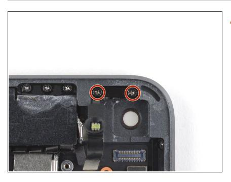
Use a Phillips screwdriver to remove the two 4.2 mm screws securing the power button bracket.
