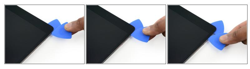
Insert a new opening pick and slide it down the right edge of the iPad, releasing the adhesive as you go.
