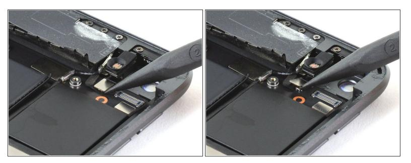
Use the pointed end of a spudger to disconnect the power button press connector.
