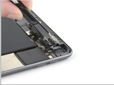
Use a pair of tweezers to remove the power button bracket.
