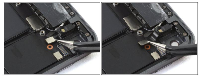
Use a pair of tweezers to pull the power button cable out from under the shelf.
