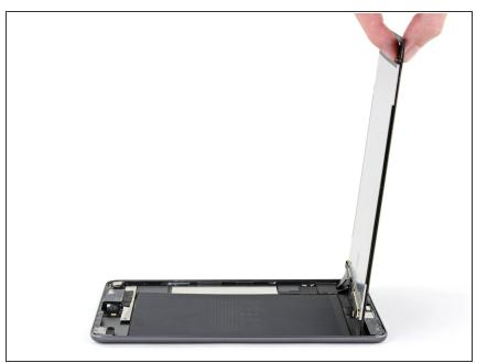
• To avoid stressing any cables, hold the screen perpendicular to the frame.
