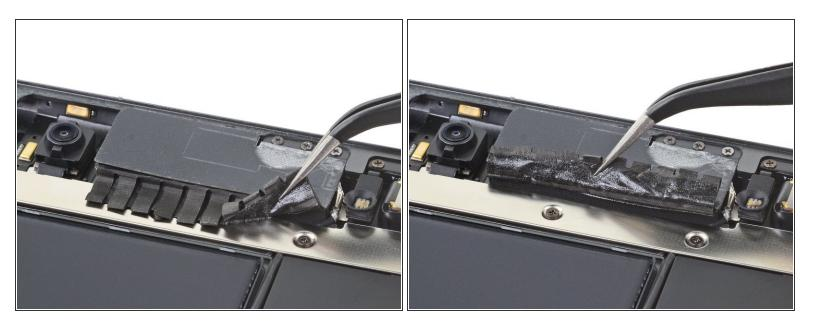
Use a pair of tweezers to lift up the tape covering the press connector cover screws.
