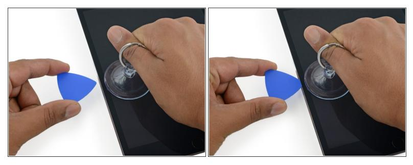
• While holding the glass up with the suction cup, insert the point of an opening pick into the gap between the glass and body of the iPad.
