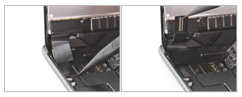
• Use the pointed end of a spudger to disconnect the digitizer press connector from the logic board.
