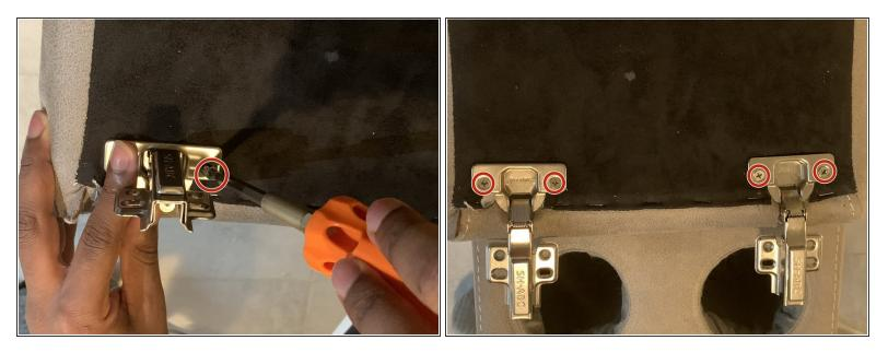
Use a Phillips screwdriver to attach each hinge to the cover of the storage compartment with two <sup>3</sup>/<sub>4</sub>-inch Flat-Head Wood screws #9.
