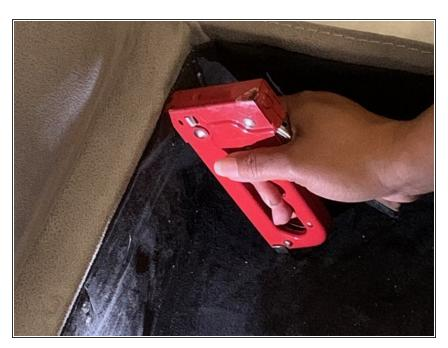
• Use the staple gun to staple the inside fabric. Allow the glued match sticks to dry for approximately 5 minutes before doing the next step.
