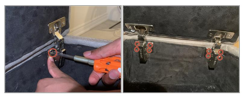
Use a Phillips screwdriver to attach each hinge to the base of the storage compartment with four ¾-inch Flat-Head Wood screws #9.
