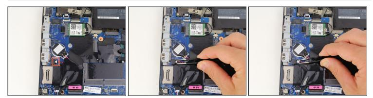
• Pull out the CMOS battery cable connector with a pair of blunt nose tweezers.
