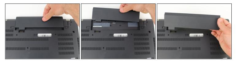
• Pull the battery directly out of the socket
