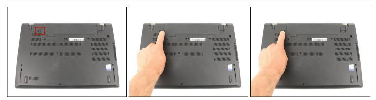
• Slide the switch on the left side of the battery to the left.
