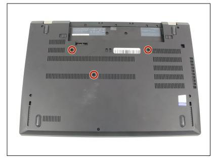
Use a Phillips #00 screwdriver to unscrew the three 3.3 mm captive screws securing the keyboard.
