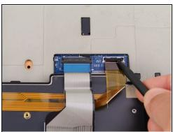
Use a spudger to lift up the two black, hinged locking flaps on the <u>ZIF connectors</u> on the motherboard.
