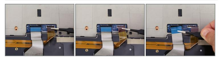
Use a pair of blunt nose tweezers to pull the two keyboard ribbon cables out from the ZIF connectors.
