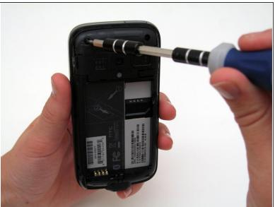
Remove the top 2 screws on the back of the phone with the T4 Screwdriver.
