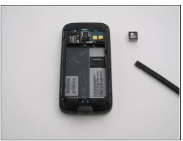
Work the metal camera casing off by slowly prying up the sides using the spudger.
