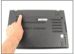
Slide the switch on the left side of the battery to the left.
