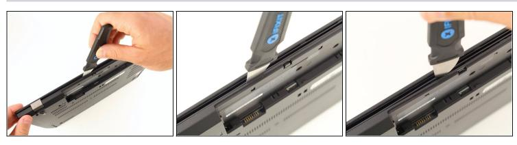
Run a Jimmy along the crease of the computer all the way around, twisting it periodically to disengage the clips.
