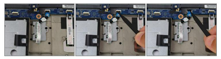
• Using a spudger, flip up the black tab of the fingerprint sensor's ZIF connector on the motherboard.
