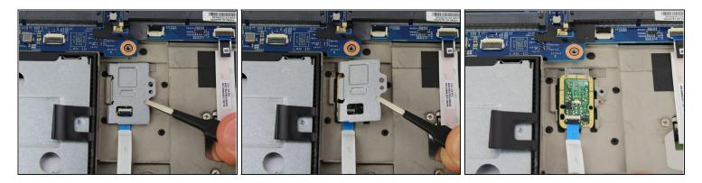
• Lift the bracket off of the fingerprint sensor board with a set of blunt nose tweezers.
