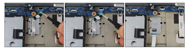
• Pull out the fingerprint sensor ribbon cable from the ZIF connector using a pair of blunt nose tweezers.
