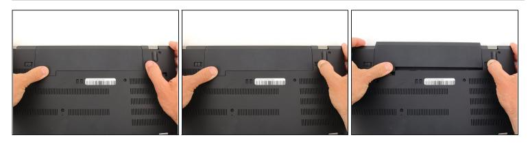
• Slide the switch on the right side of the battery to the right while applying upward pressure on the battery.
