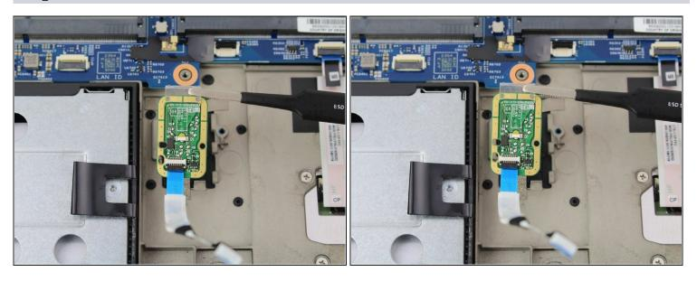
• Lift the fingerprint sensor out from the device with a pair of blunt nose tweezers.
