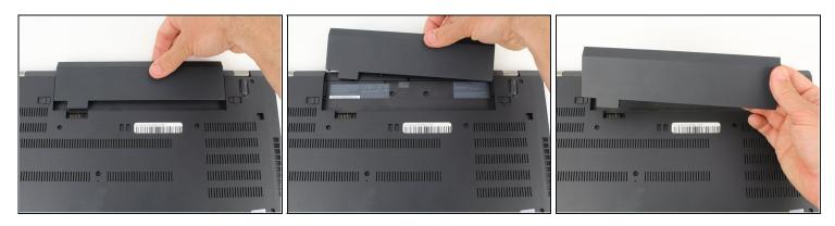
• Pull the battery directly out of the socket
