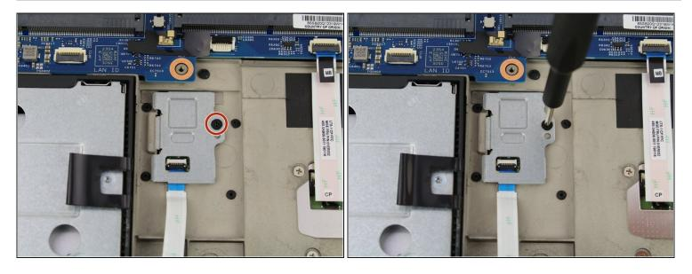
Using a Phillips #00 screwdriver, remove the 3.0 mm screw from the fingerprint sensor bracket.
