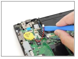
Using the plastic opening tool, disconnect the CMOS battery from the motherboard.
