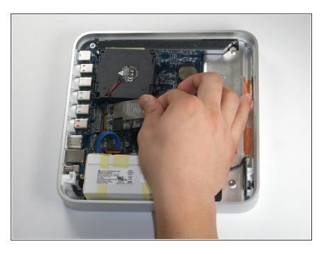
Cautiously lift the AirPort card and pull it straight away. Slide it from its socket on the logic board.
