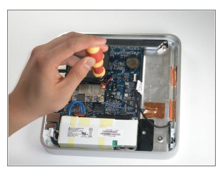
Remove the single T8 Torx screw securing the AirPort card to the logic board.
