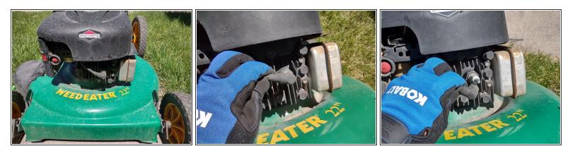
Disconnect the spark plug wire and tuck it away from the spark plug to avoid any accidental startups.
