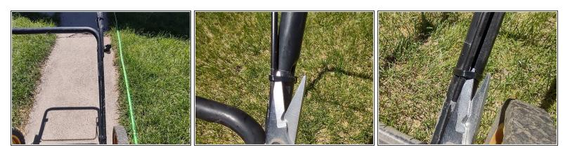
Use the utility shears to cut the zip ties which secure the cable to the upper and lower handles of the mower.
