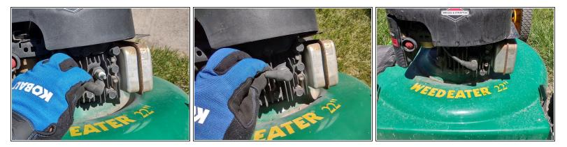
• Reconnect the spark plug wire to the spark plug.
