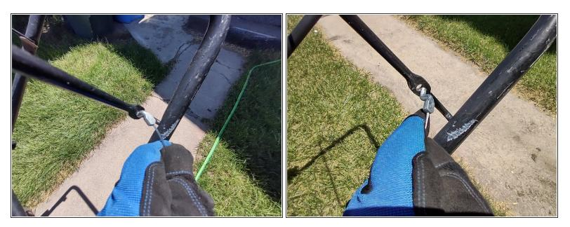
• Attach the cable to the control bar by pushing the Z end of the cable into the hole.
